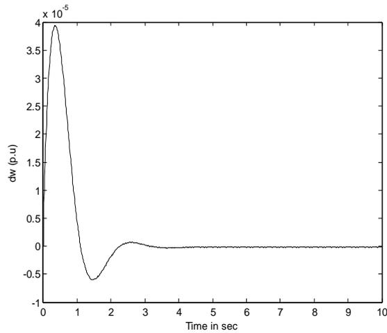
Fig. 7: Response of speed deviation ( $\Delta\omega$ ) for  $m_1$  of IPFC controller with Lead-Lag controller
