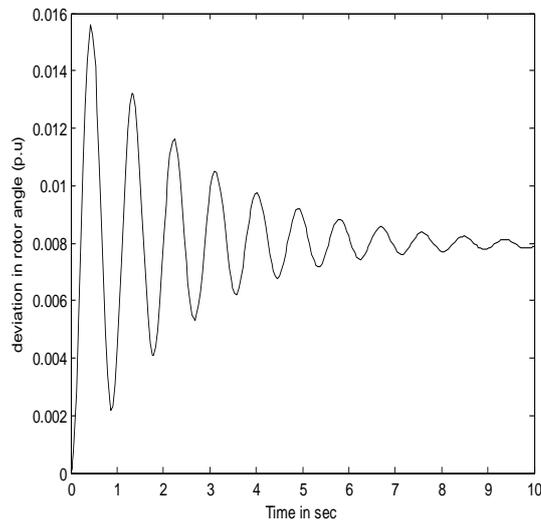
Fig. 14: Response of rotor angle deviation ( $\Delta\delta$ ) for  $\delta_2$  of IPFC controller with Lead-Lag controller
