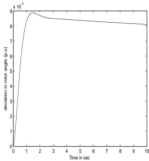
Fig. 12: Response of Rotor angle deviation ( $\Delta\delta$ ) for  $m_2$  of IPFC controller with Lead-Lag controller
