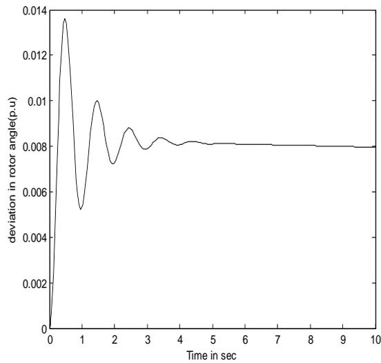
Fig. 10: Response of Rotor angle deviation ( $\Delta\delta$ ) for  $\delta_1$  of IPFC controller with Lead-Lag controller
