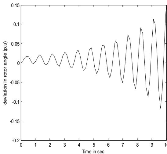
**Fig. 6: Response of Rotor angle deviation ( $\Delta\delta$ ) without any supplementary controller**
