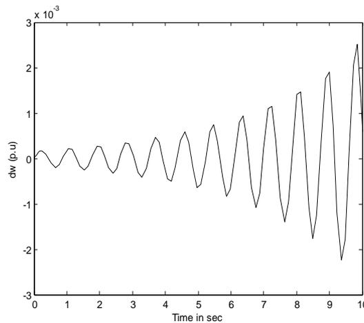
**Fig. 5: Response of speed deviation ( $\Delta\omega$ ) without any supplementary controller**
