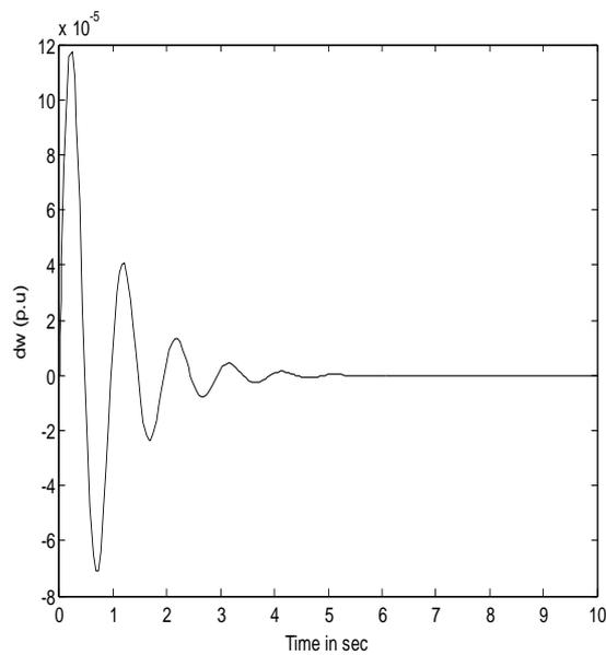
Fig. 9: Response of speed deviation ( $\Delta\omega$ ) for  $\delta_1$  of IPFC controller with Lead-Lag controller
