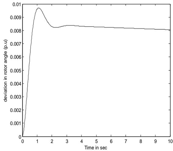
Fig. 8: Response of Rotor angle deviation ( $\Delta\delta$ ) for  $m_1$  of IPFC controller with Lead-Lag controller
