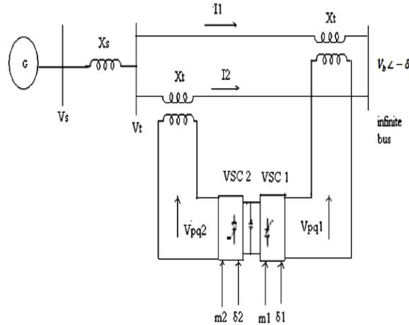
Fig.1: Single Machine Infinite Bus installed with IPFC
