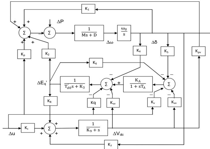
Fig. 2 : PH model of SMIB system installed with IPFC
