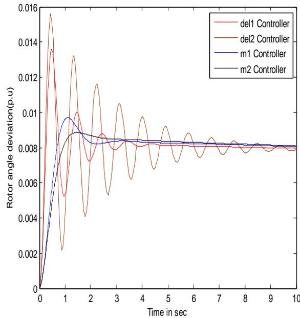
Fig. 16: Response of rotor angle deviation ( $\Delta\delta$ )
