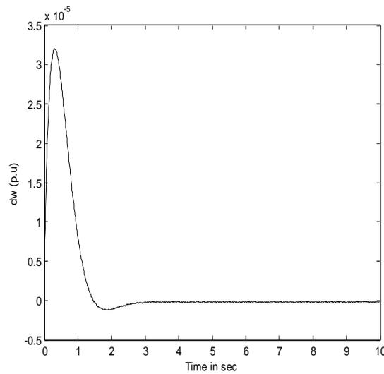
Fig. 11: Response of speed deviation ( $\Delta\omega$ ) for  $m_2$  of IPFC controller with Lead-Lag controller
